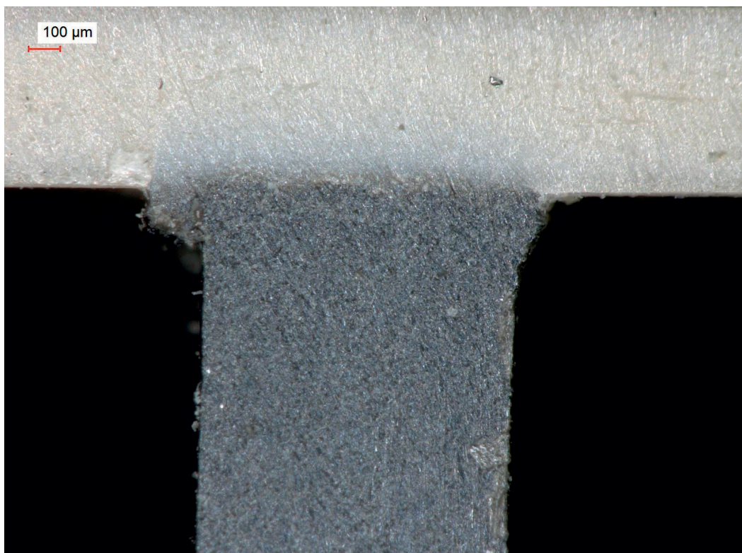
Cross-section of a weld seam: The microsection of the seam shows a joining zone and characteristic melt flow for quasi-simultaneous welding © Evosys, DIC
